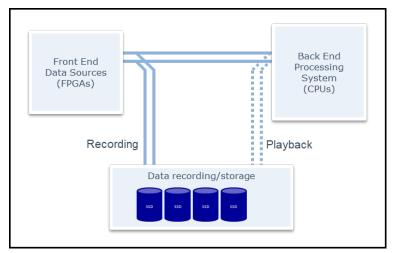
Without the recording requirement, 10GbEthernet with UDP would probably be the best solution (section 5.1.1 review below), provided that the system has reliable link connectivity (so the link error rate is very low, and resend or guaranteed delivery is not required).
