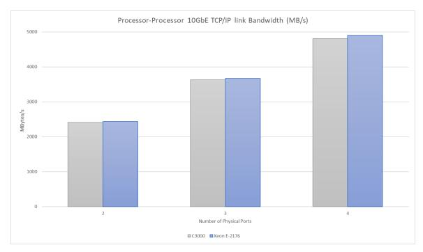
The above chart shows that for both processors (and associated NICs), the TCP/IP overhead is minimal. Link utilization figures are over 96% even with 4 physical ports active simultaneously. This is only possible because offload engines are dealing with the TCP/IP protocols.
