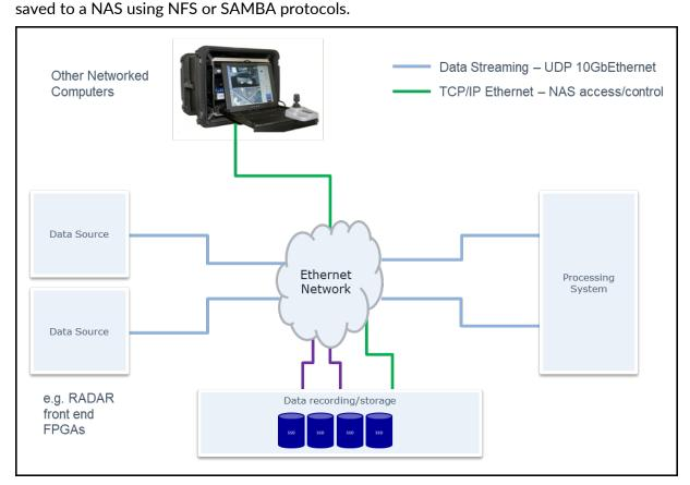
One issue with these high level protocols for real time data transfer is timing uncertainty. Typically TCP/IP is used as a lower layer, with its advantages of guaranteed packet delivery, resend, etc. The higher level protocols implement further protections, for instance around shared resources and authentication. Timing is not necessarily predictable or repeatable. E.g. if a CRC check fails, and resend occurs, then transfer timing becomes effectively non-deterministic.
