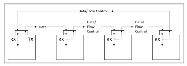
The original release of VITA 17.1 (sFPDP Gen 1.0) supported three different bit rates up to 2.5Gbaud, and 8b/10b encoding (i.e. data flow could occupy up to 80% of the bit rate). Galleon extended the use of sFPDP from the 2.5Gbaud maximum defined in the standard up to 4.25Gbaud. The VITA 17.1 standard was extended up to 10Gbaud in the most recent update, ratified in 2015.
