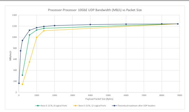
Although UDP is a much simpler protocol than TCP/IP, the processor must deal with the protocol directly, so small packet sizes can have a large impact on the achievable bandwidths. If there are a small number of logical ports, then some of the Ethernet FIFOs/buffers and processor threads cannot be used (for the single threaded application), further limiting the performance.
